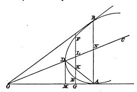
1st. Let the given point D be in ON; then, if ND = OD, the curve is a parabola.
